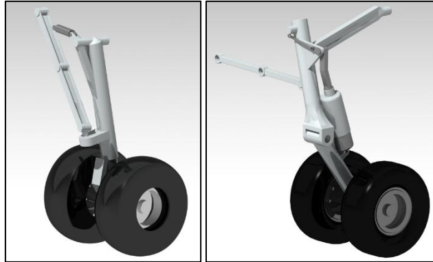
Figure 2. Ae-16 landing gear solutions (left: wing-mounted telescopic; right: fuselage-mounted trailing arm)
