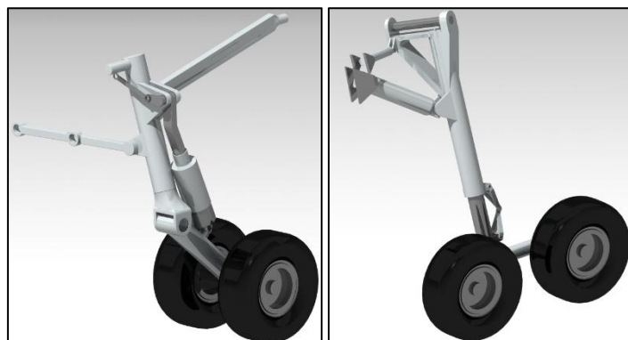
Figure 3. A-17 landing gear solutions (left: trailing arm; right: telescopic)
