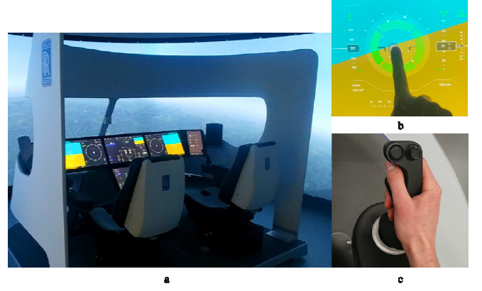
Fig. 1. Cranfield University/Rolls-Royce FSS (1a) with the touchscreen inceptor integrated into the middle of the primary flight display (1b) and traditional sidestick controller as the baseline operational mode (1c)
