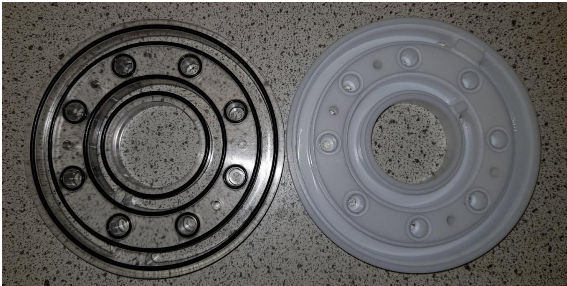
Figure 3.9 Meso scale OBR disks with spiral heating/cooling channels (Acrylic and PTFE materials)
