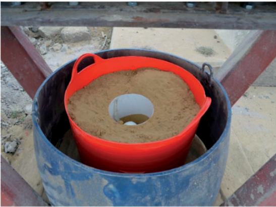
Figure 4. Contained sand with centre location excavated to enable placement of PE4.
