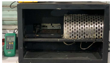
Figure 1. A schematic diagram and photo of the apparatus for experimentation of single droplet combustion.
