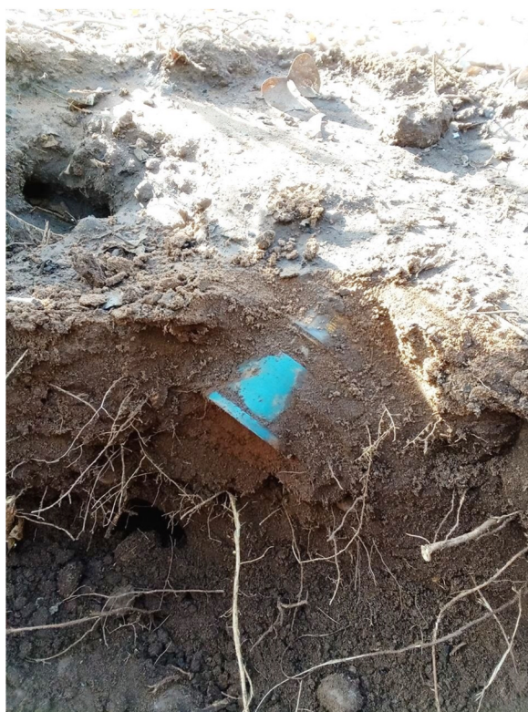
Fig. 2. Item_Report-240309125917 of the trial photographed once excavated. The mine was estimated to have tilted 35^\circ . The blue 100g TNT booster is clearly the visible. The deminer has excavated the mine no more than necessary to identify it and place a donor charge. (For interpretation of the references to colour in this figure legend, the reader is referred to the Web version of this article.)
