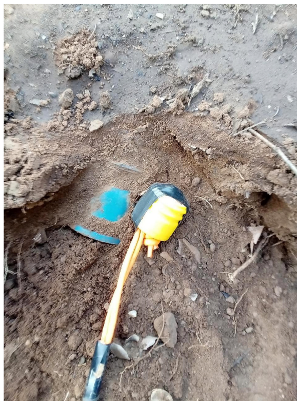
Fig. 3. A 37.5g pentolite donor charge placed next to the mine.
