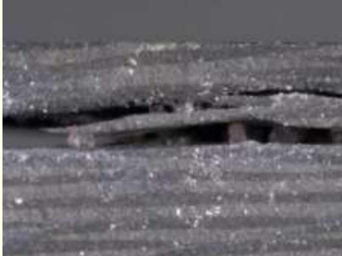
Figure 1. Delamination failure in a CFRP laminate.
