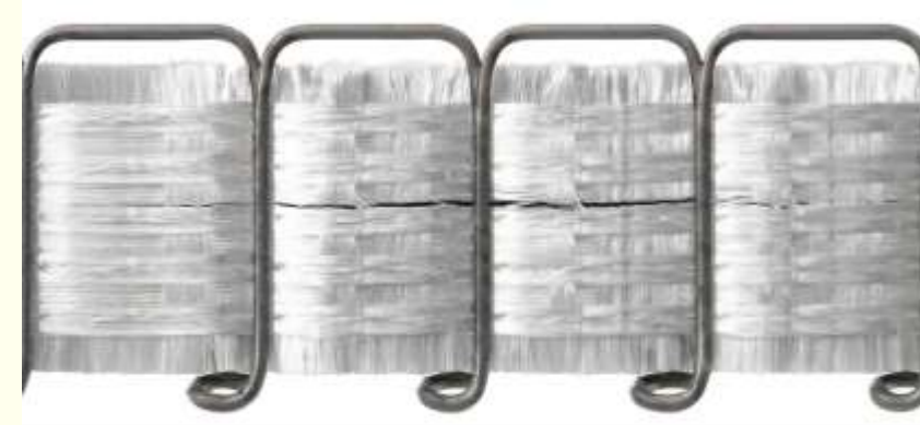
Figure 3. Cracked composite matrix prior to healing activation.
