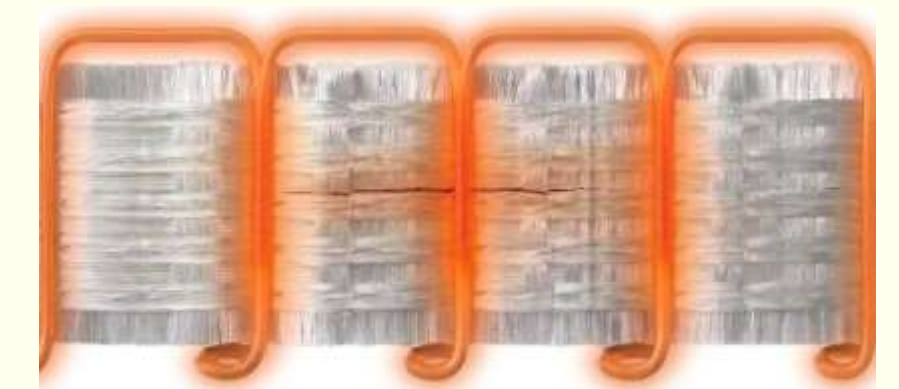
Figure 4. Resistive heating via electrical current through the nichrome tuft.
