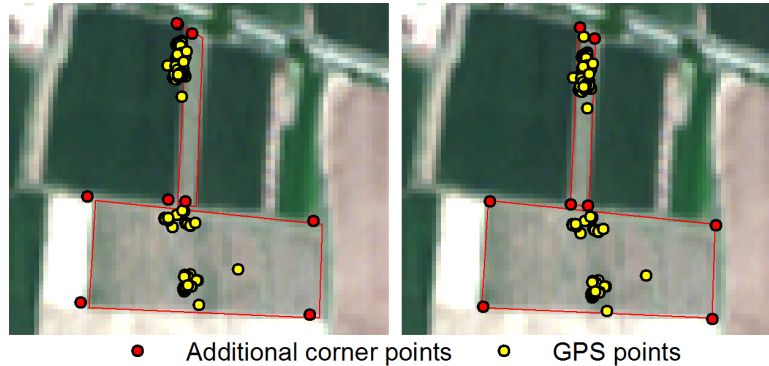
Figure 3: Suggested additional GPS point locations at field corners allow improved placement of yield points with imagery. GPS points shifted to image (right) using field corners.
