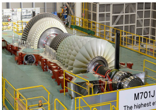
Fig. 1. Heavy-duty gas turbine
