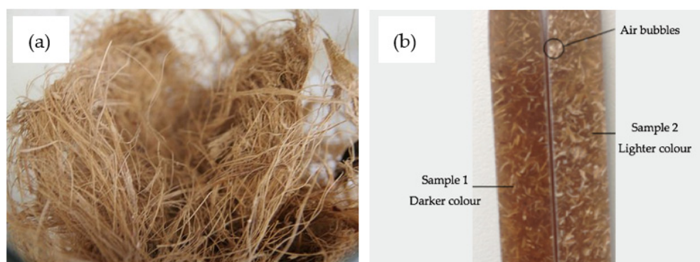
Figure 9. (a) Example of as-received agave bagasse waste for laboratory scale experiments. (b) Example of the preliminary resulted material prototype agave fibres and PLA.
