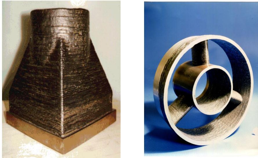
Figure 6.1.1 Nickel alloy components for flight applications [Image taken from a presentation by Prof John Norrish]
