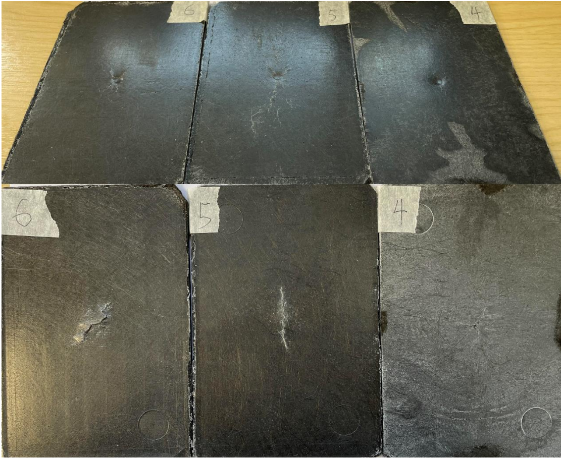
Figure 28. Top and rear side image of RCF & powder PP samples after impact
