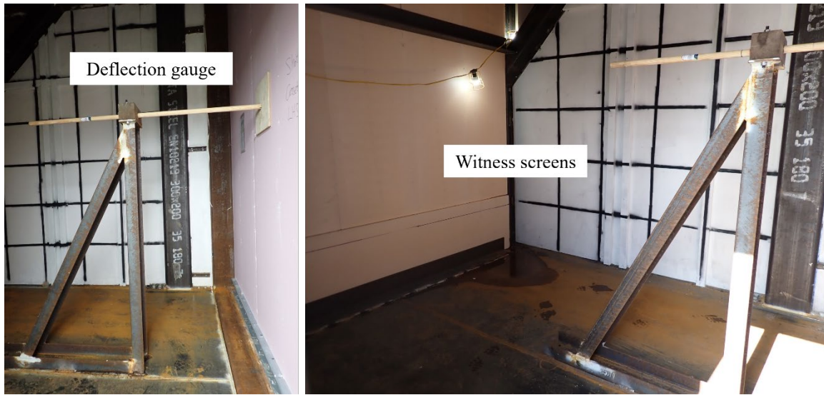
Figure 6 Deflection gauge and witness screens behind each target
