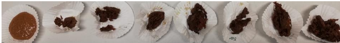
Fig-8: From left to right: samples of simulant sludge after a) 0, b) 30, c) 35, d) 40, e) 45, f) 50, g) 55, h) 60 minutes of drying
