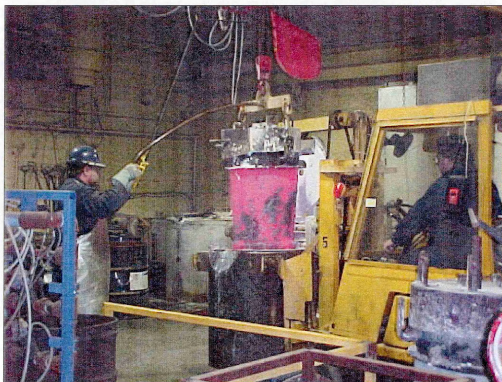
Figure 34 Lowering crucible into pouring lift-truck.
