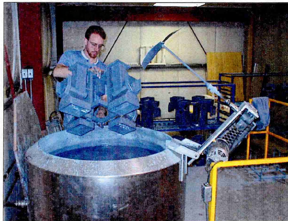
Figure 11, Figure 12 Assembly and coating of pattern (Inmetalna, 2000).
