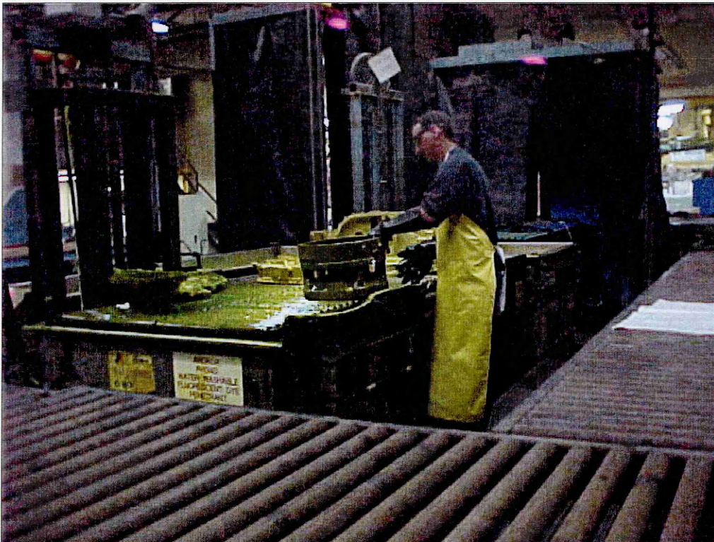
Figure 50 Draining fluorescent penetrant oil from casting.
