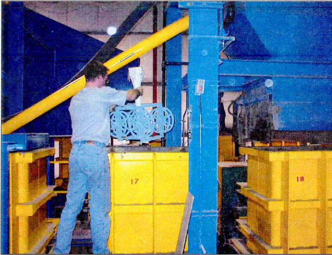
Figure 13 Placing pattern in the flask (Inmetalna, 2000).
