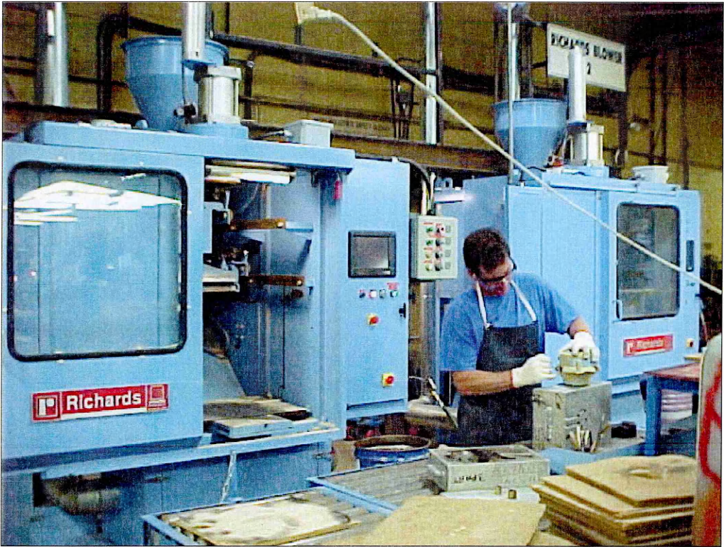
Figure 27 Cold box coremaking machines.
