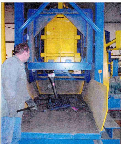
Figure 15 Removal of casting from moulding material (Inmetalna, 2000).
