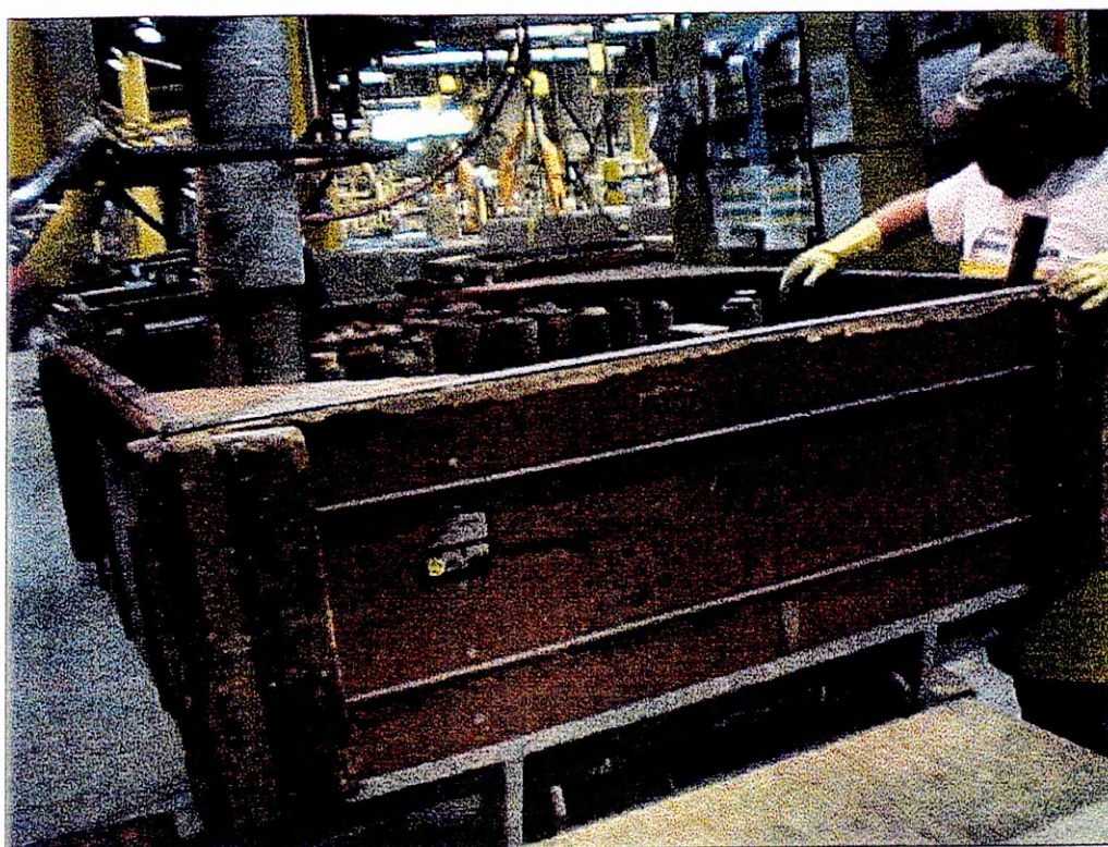
Figure 2 Filling pattern box with sand.
