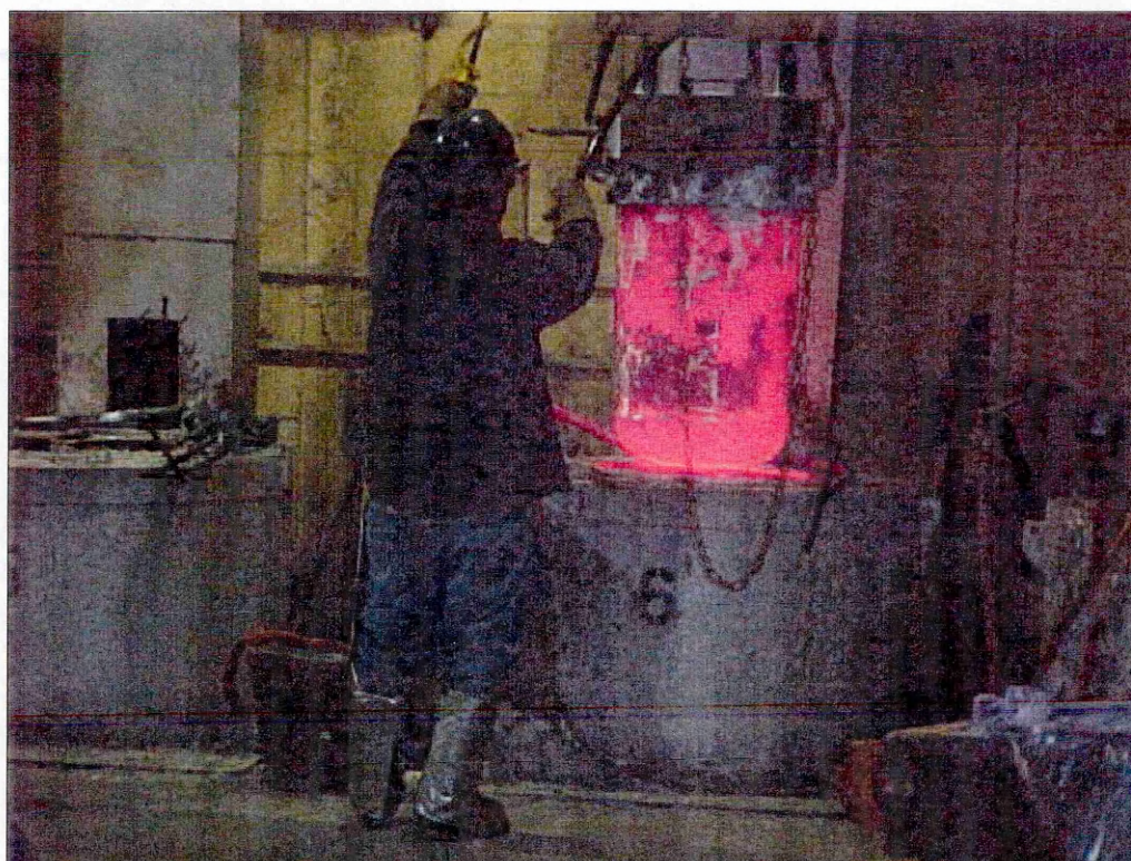
Figure 33 Lifting a crucible of magnesium from the furnace.
