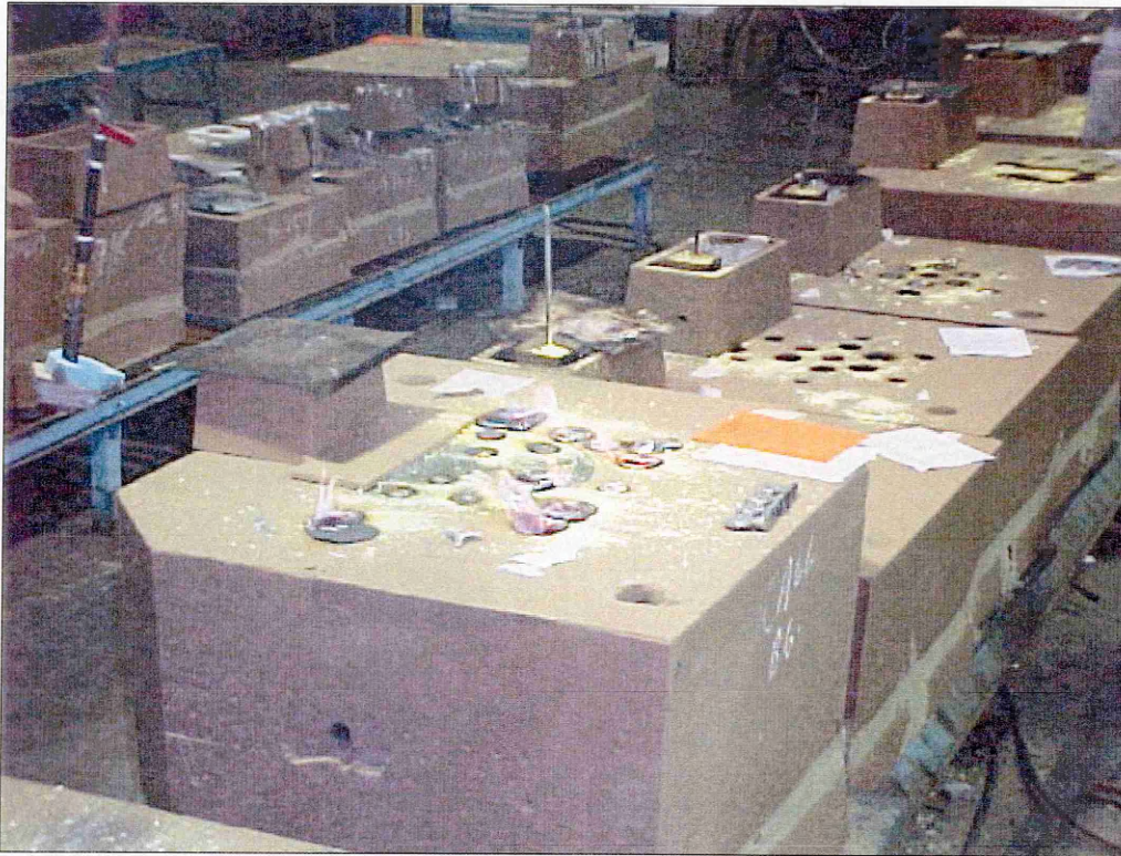
Figure 36 Moulds after pouring.
