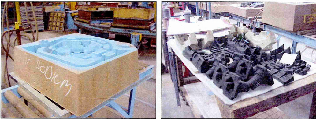
Figure 20, 21 Mould and cores awaiting assembly.
