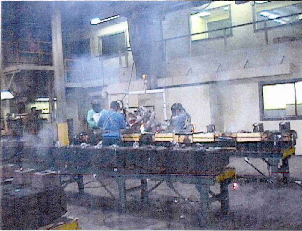
Figure 6 Pouring green sand moulds at Presto Castings.
