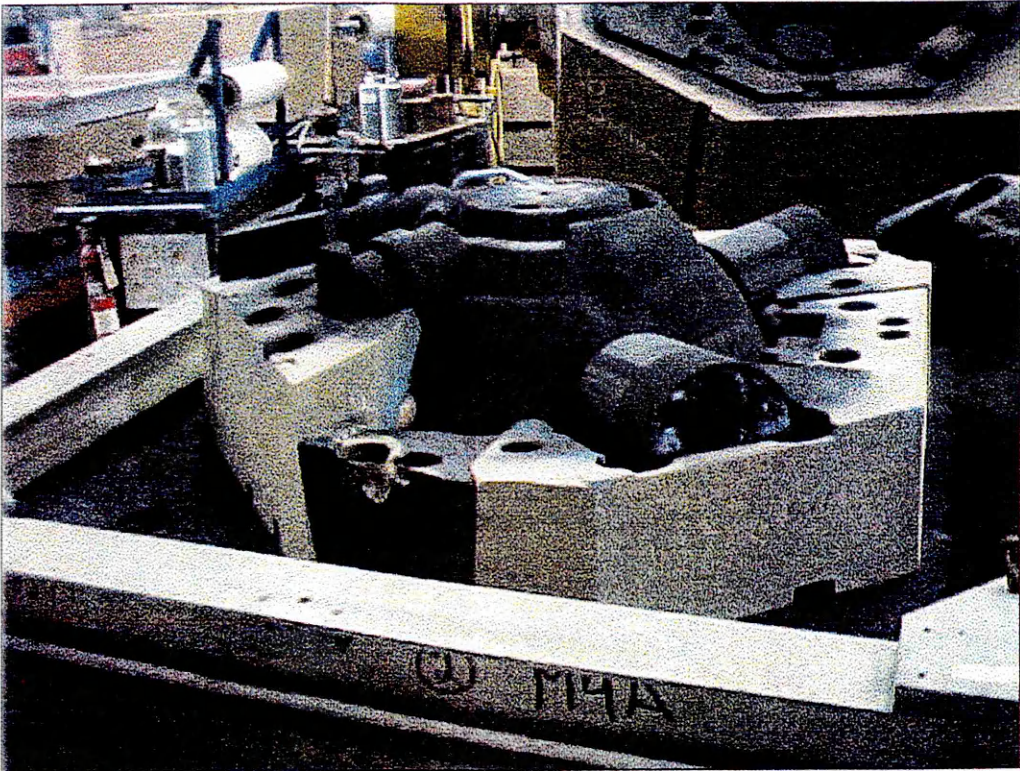
Figure 6 70351-38111 cope during assembly.
