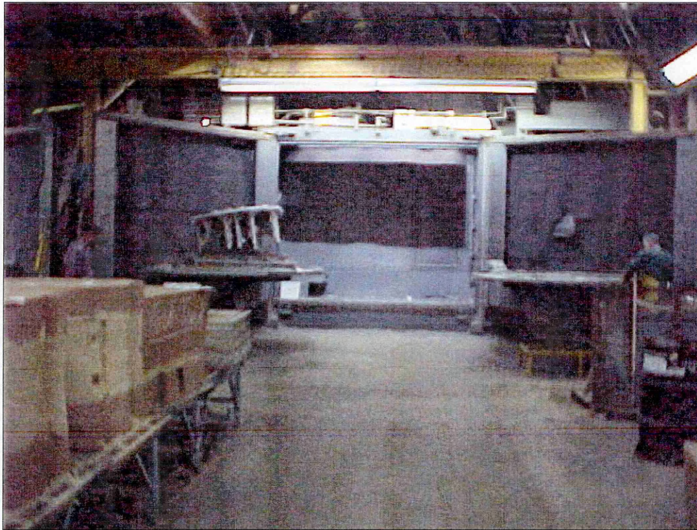
Figure 38 Shot-blast unit for sand removal from casting.
