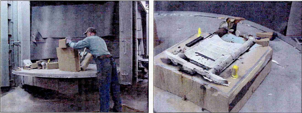
Figure 11, 12 Breaking casting away from the mould.
