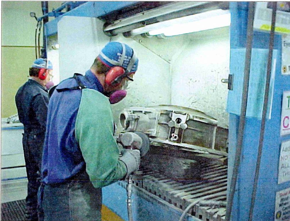
Figure 46 Disk sanding a casting.
