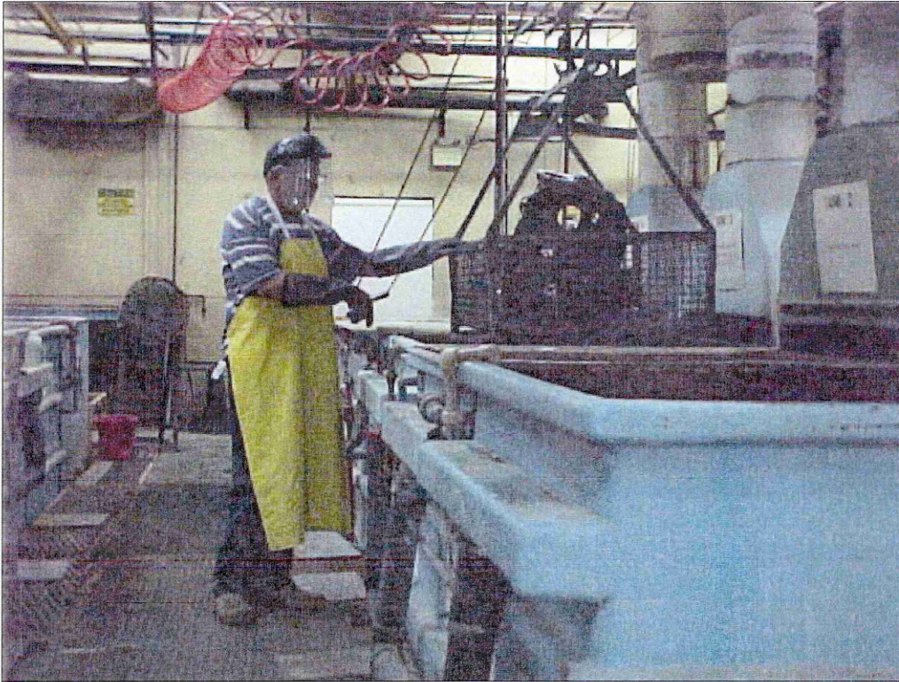
Figure 49 Acid etching castings before inspection.
