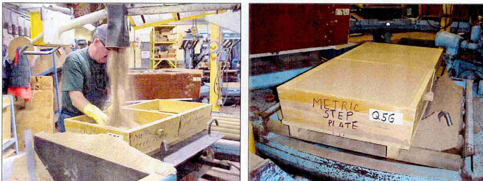
Figure 3, 4 Mould packing and curing.
