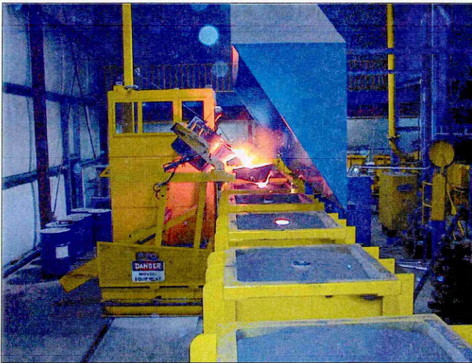
Figure 14 Pouring metal into the mould (Inmetalna, 2000).
