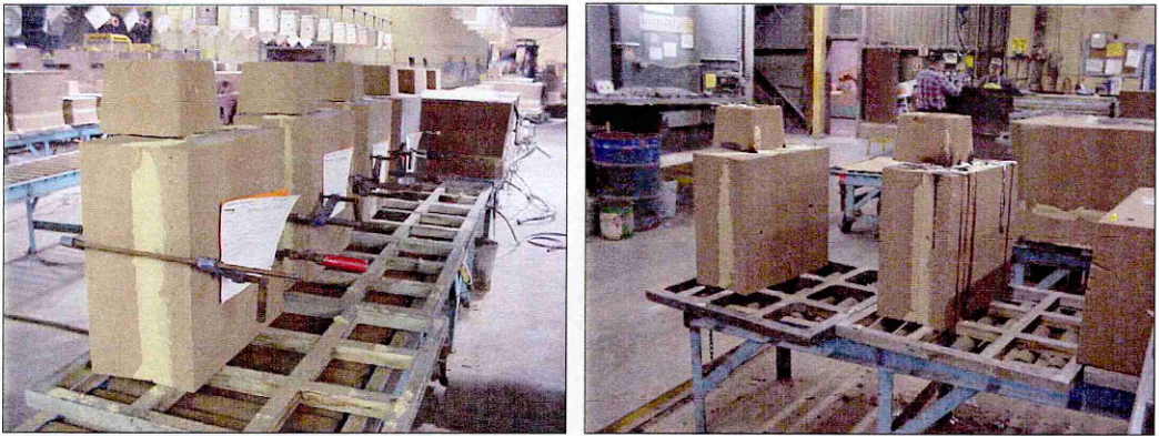
Figure 9, 10 Moulds before and after pouring.
