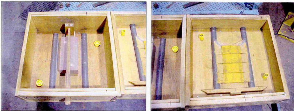
Figure 1, 2 Test plate pattern, cope side (left) and drag side (right).
