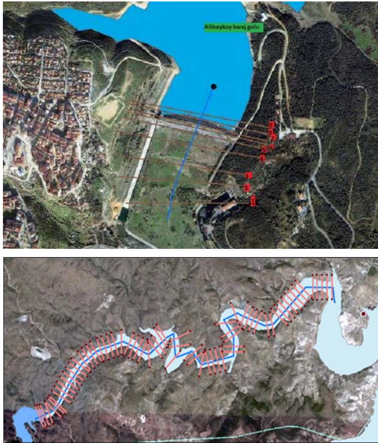
Figure 6. Cross sections used in modeling of 1 D flow of flood propagation via HEC-RAS along the Alibey and Porsuk creeks after the dam-break
