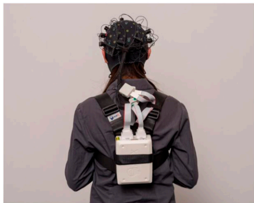
Figure 3. fNIRS equipment. In our experiment, we attached the backpack to the back of the driver's seat. Source: nirx.net .
