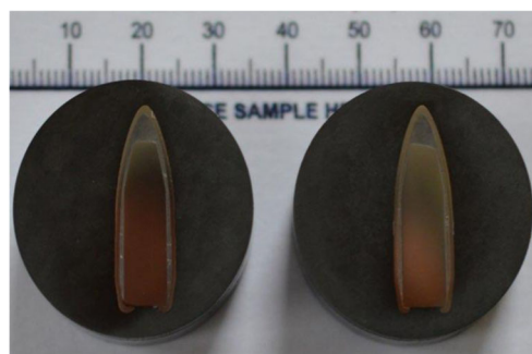
Fig. 1 Sectioned 7.62 × 39 mm bullets. Left , Czech; right , Ukrainian
