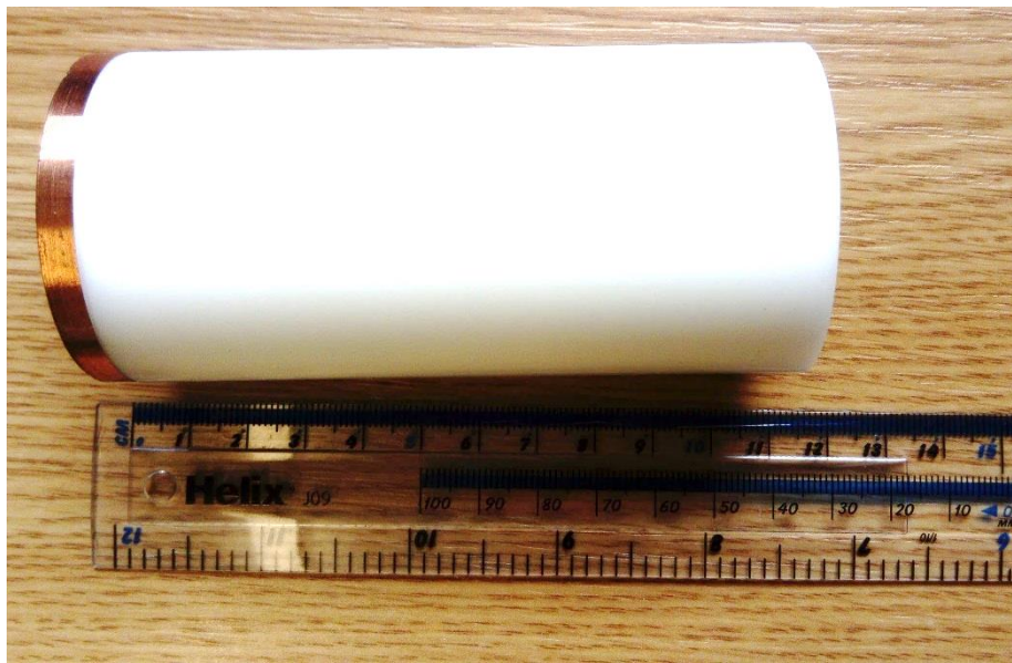
Figure 25: 10 mm copper flyer plate attached to POM sabot
