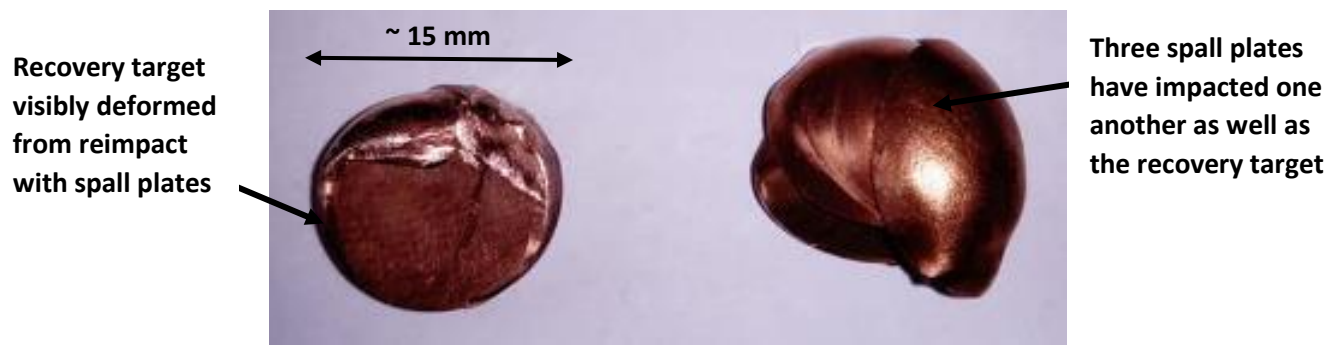
Figure 51: Spall plates having reimpacted the recovery target
