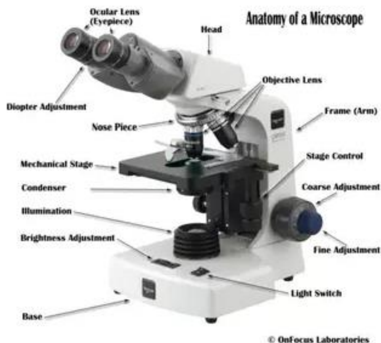
Figure 37: Labelled compound light microscope (©OnFocus Laboratories)
