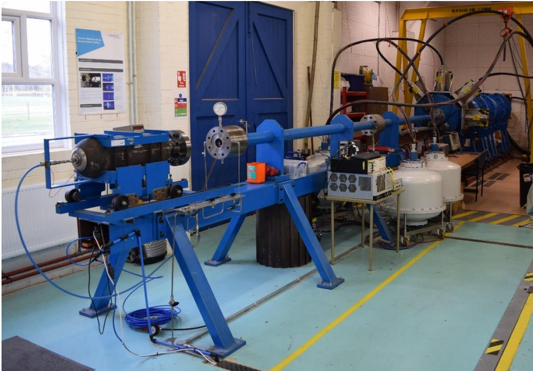
Figure 18: Image of a 50 mm bore, 6 m long single-stage gas gun
