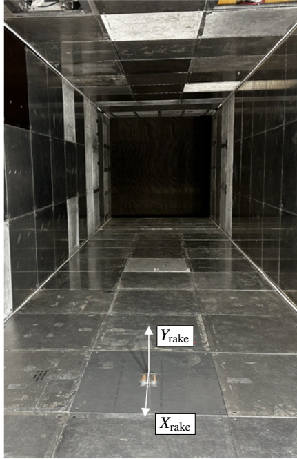
(c) Floor-mounted boundary-layer rake.
