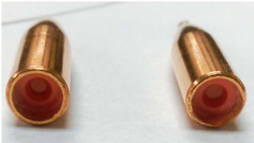
Figure 1-1 M276 round example (red is the igniter shielding the fuel and oxidiser) [1]
