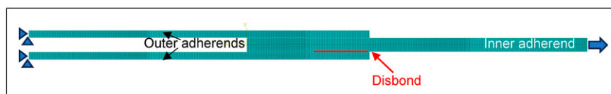
Figure 15. FE mesh and boundary conditions.
