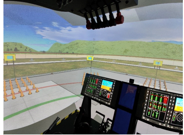
Figure 8: Cockpit view of XWH low-speed controllability ACR simulator set-up in UoL's HELIFLIGHT-R simulator (Ref. 29).
