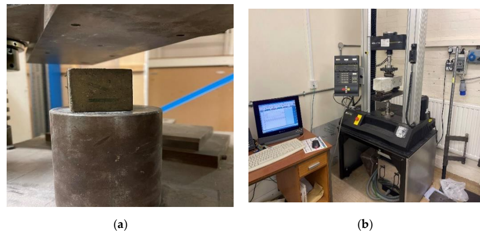
Figure 3. Mechanical tests. (a) Compressive strength test. (b) Flexural strength test.
