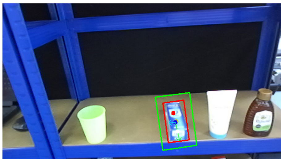
Figure 7. PCA ambiguity in angle prediction, while the red dot is enhanced point from PCA to calculate aspect ratio together with the blue dot, which is centroid point. The arrows show primary and secondary axis.
