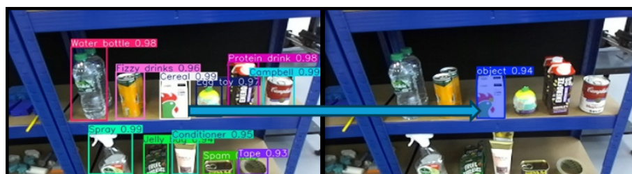
Figure 3. From object detection to instance segmentation (FAST-SAM).
