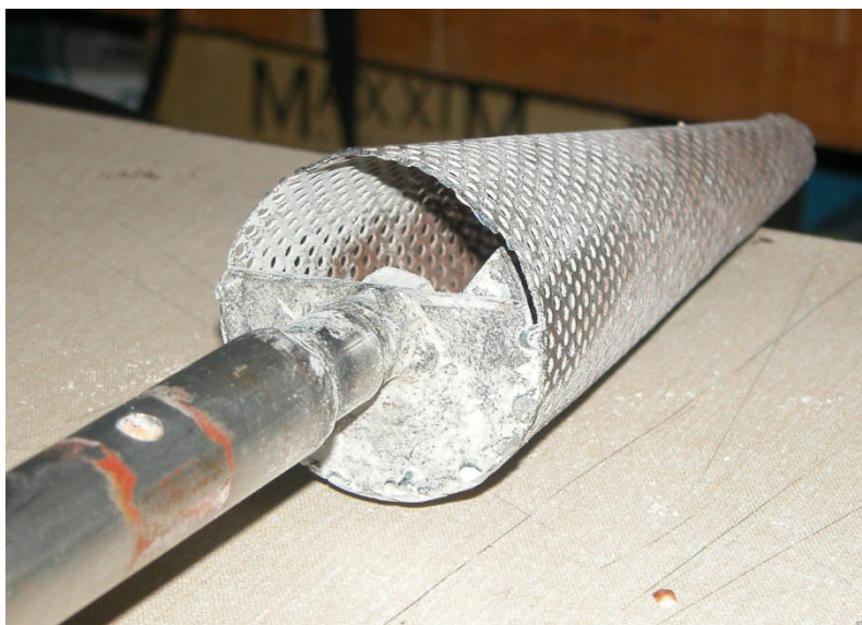
Figure 2. Detail of the chamber on the sampling probe in the open position
