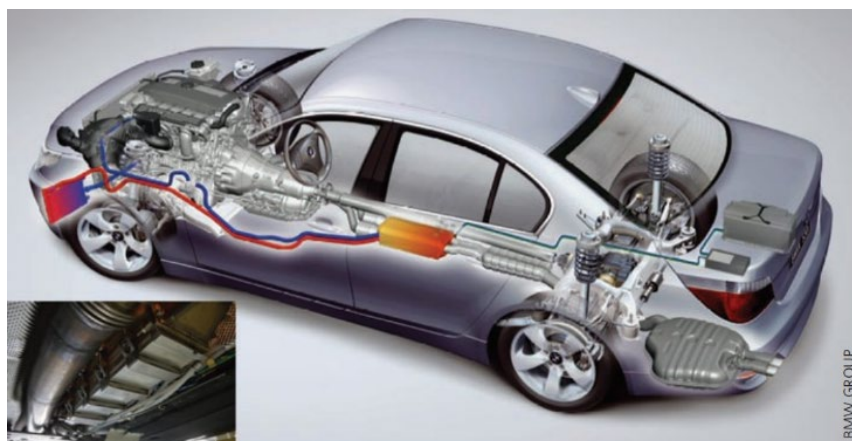
Figure 2-12 integrating thermoelectrics into vehicles for improved fuel efficiency (C. B. Vining, 2009)
