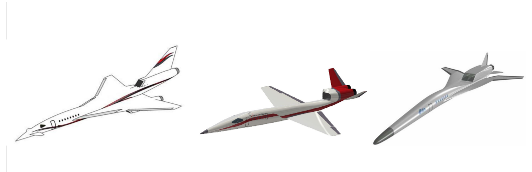
Figure 15. HISAC project concepts for low noise ( left ), long range ( center ) and low boom ( right ). (Source: [144].)
