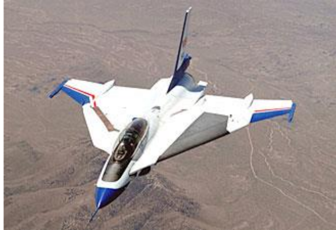
Figure 4.4 The F16xl in boundary layer control experiment [35]
