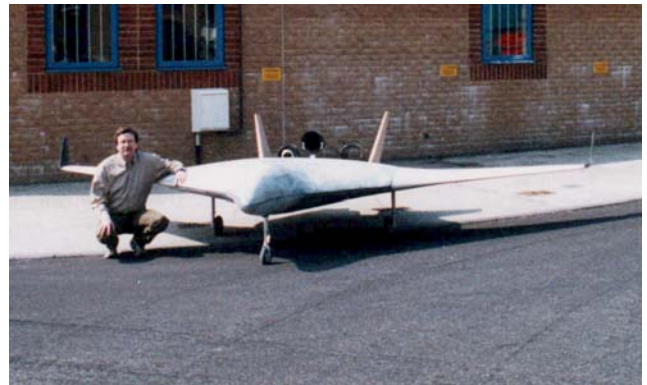
Fig 2: Kestrel BWB Demonstrator UAV
