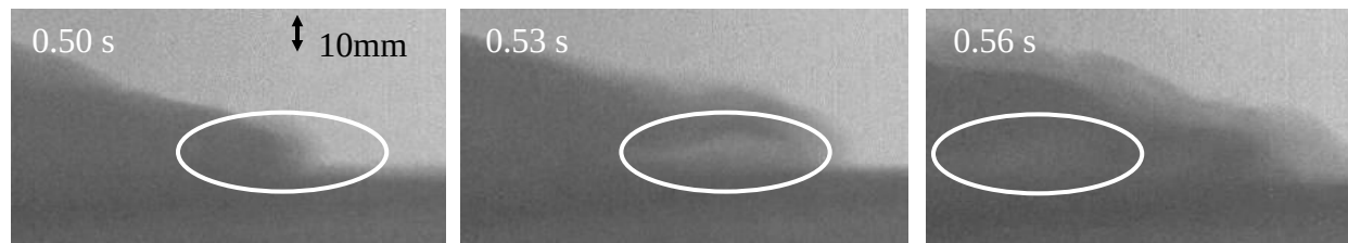
Figure 8. Instability in advancing flow front leading to entrainment of an air bubble; Trial 2
