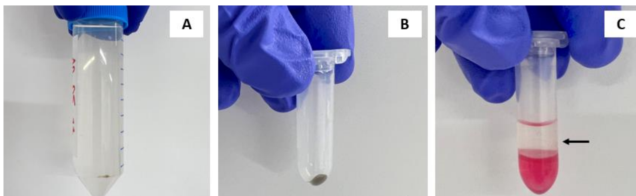
Figure 3-2: Wastewater concentration by PEG-Precipitation. (A) Centrifuged sample after overnight incubation. (B) Pellet obtained prior to TRIzol resuspension. (C) Phase separation following TRIzol and Chloroform addition. Arrow pointing to the RNA layer.
