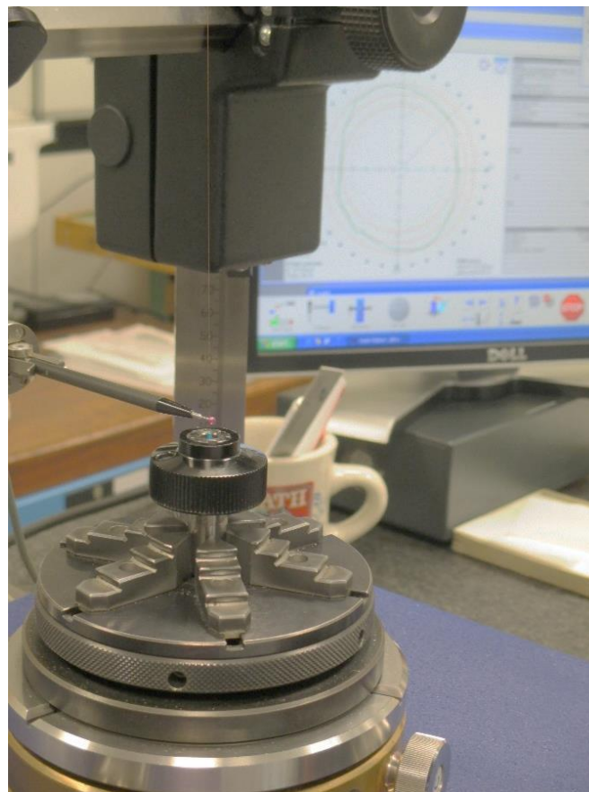
Figure 9-11: Contacting measurement aiming to evaluate the wire roundness
