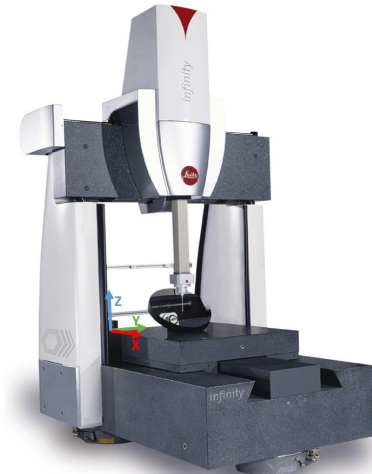
Figure 1-7: Leitz Infinity Coordinate Measuring Machine the table moves along the X-axis, the vertical column ranges the Z-axis while it scans the Y-axis carried by the horizontal bridge
