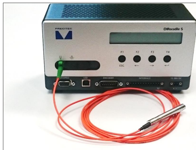
Figure 4-11: White light chromatic confocal sensor and its CHrocodile S controller
