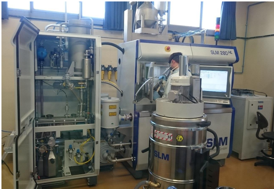
Figure 7-4: The SLM 280 HL machine with the operator during powder removal of the SESHAT's rotor
