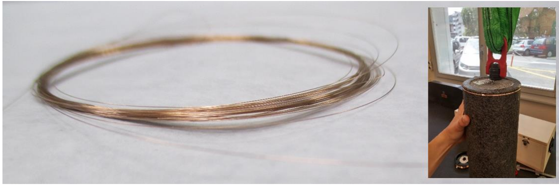
Figure 9-6: Roll of 7.540 m of copper-beryllium wire obtained by winding it around a cylinder gauge, to be weighted by a chemistry scale
