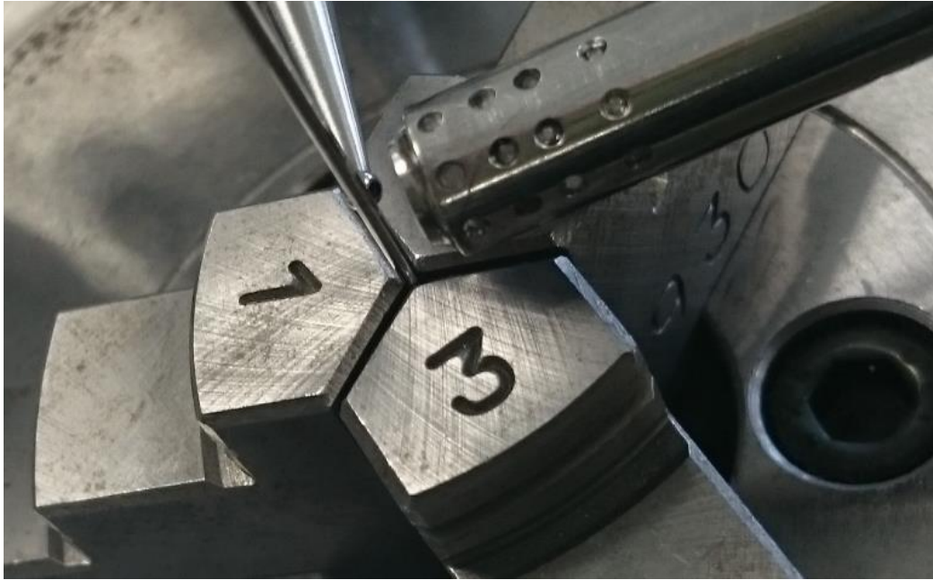
Figure 4-13: Chromatic confocal sensor versus contact measurement on a 1 mm in diameter cylinder gauge (top-down view).
