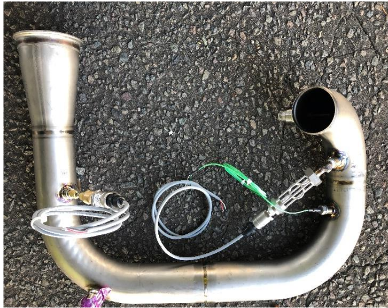
Figure 3-5 SHX inlet duct with sensors installed
