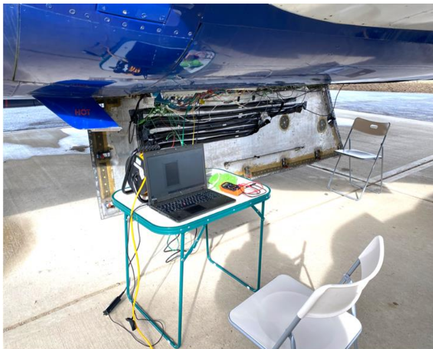
Figure 4-5 Ground test facility of the Boeing 737-400, Left-side PACK data collection
