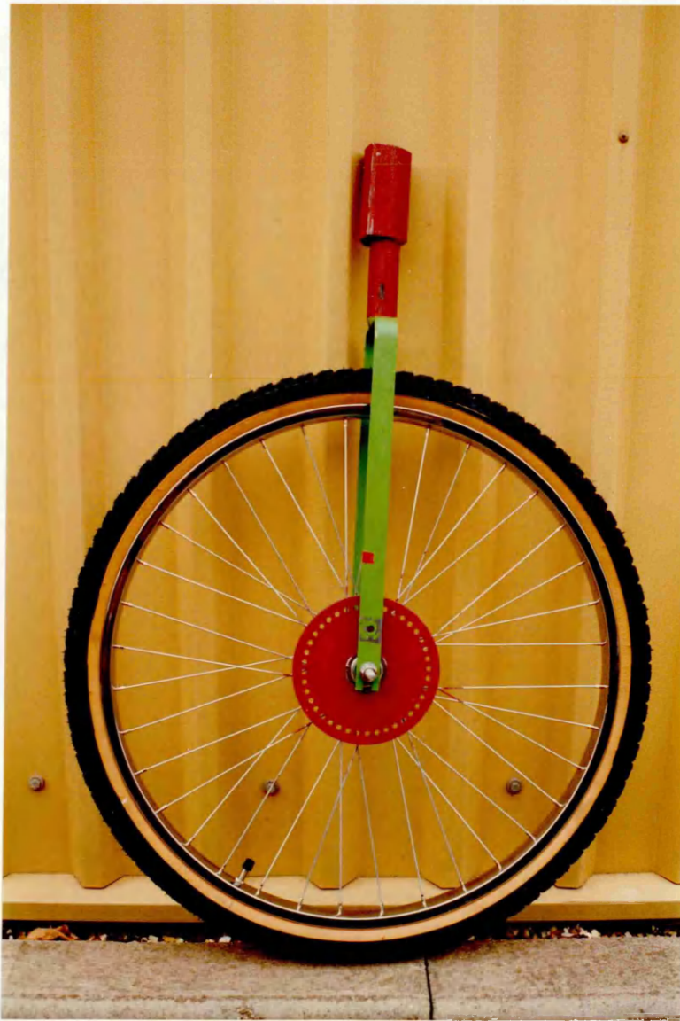
Plate 4.10. A 26 inch bicycle wheel used in the fifth wheel unit
