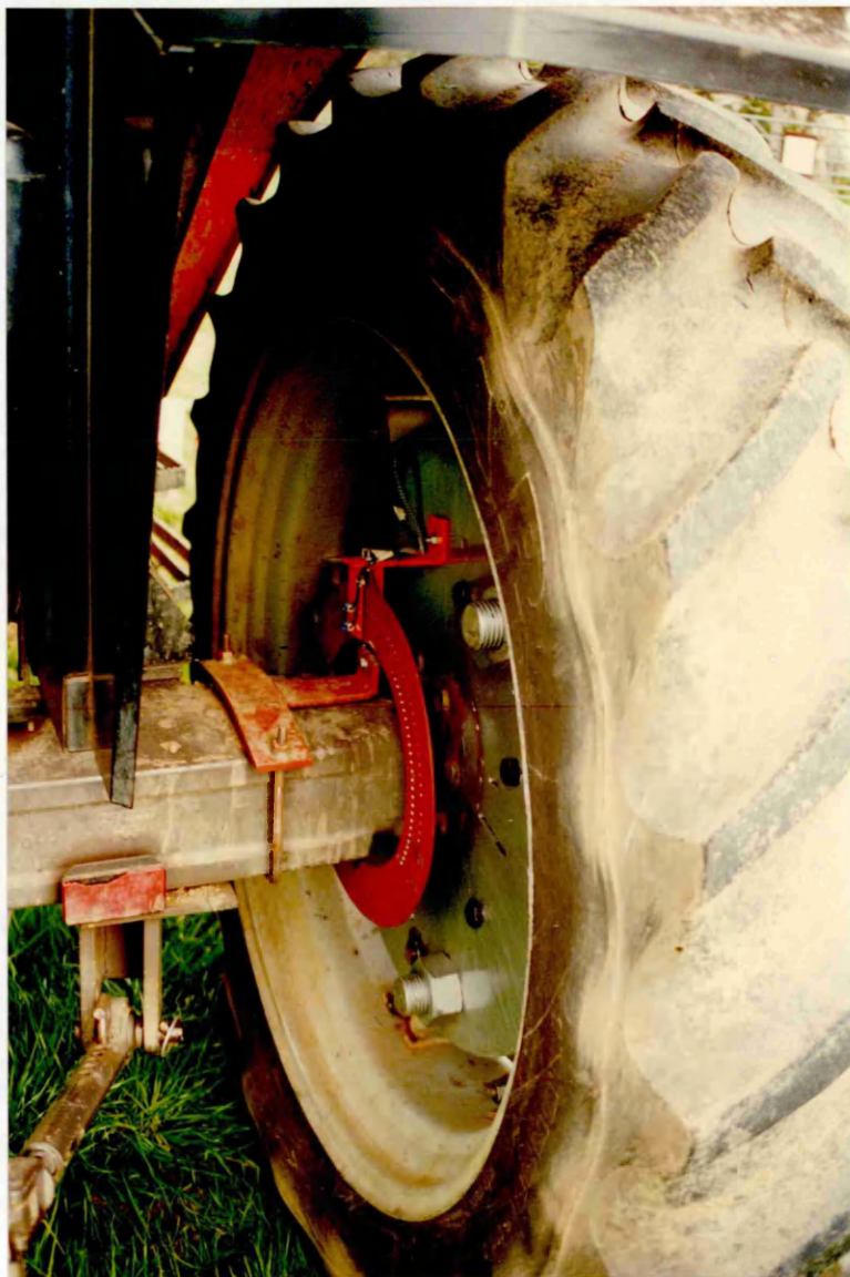
Plate 4.15. Sensors and multi-holes ring fitted to the instrumented rear wheel
