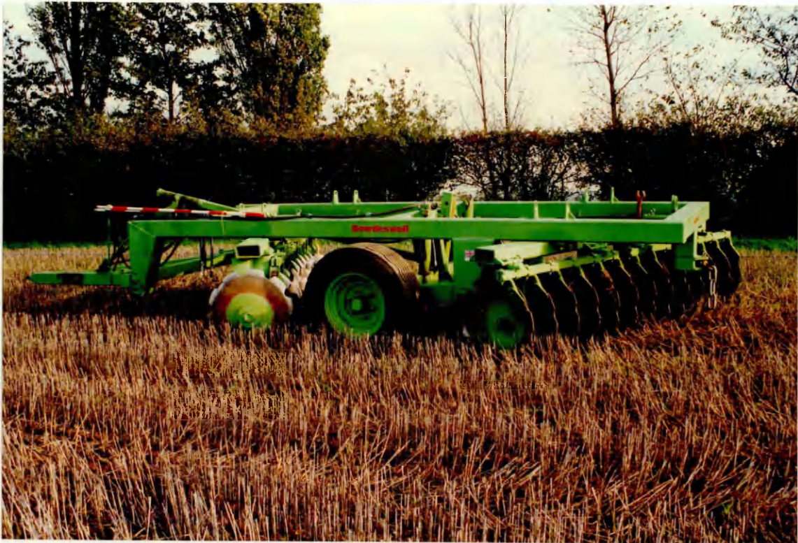
Plate 5.1. Disc Harrow (the implement used)
