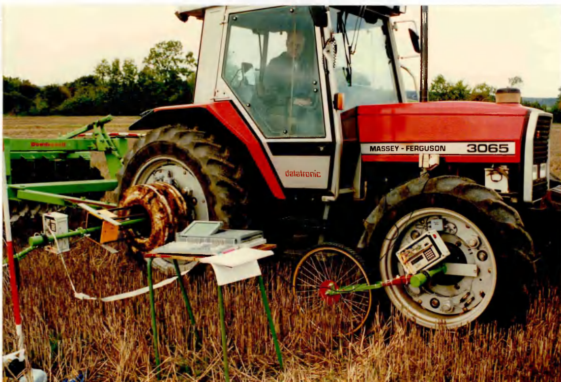
Plate 5.11. Arrangement of down loading the datalogger program to the system
