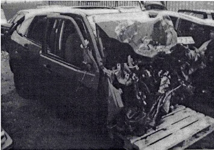
Figure 57. A real world crash with a high delta-v and a fully distributed deformation (Kirk, 2002).
