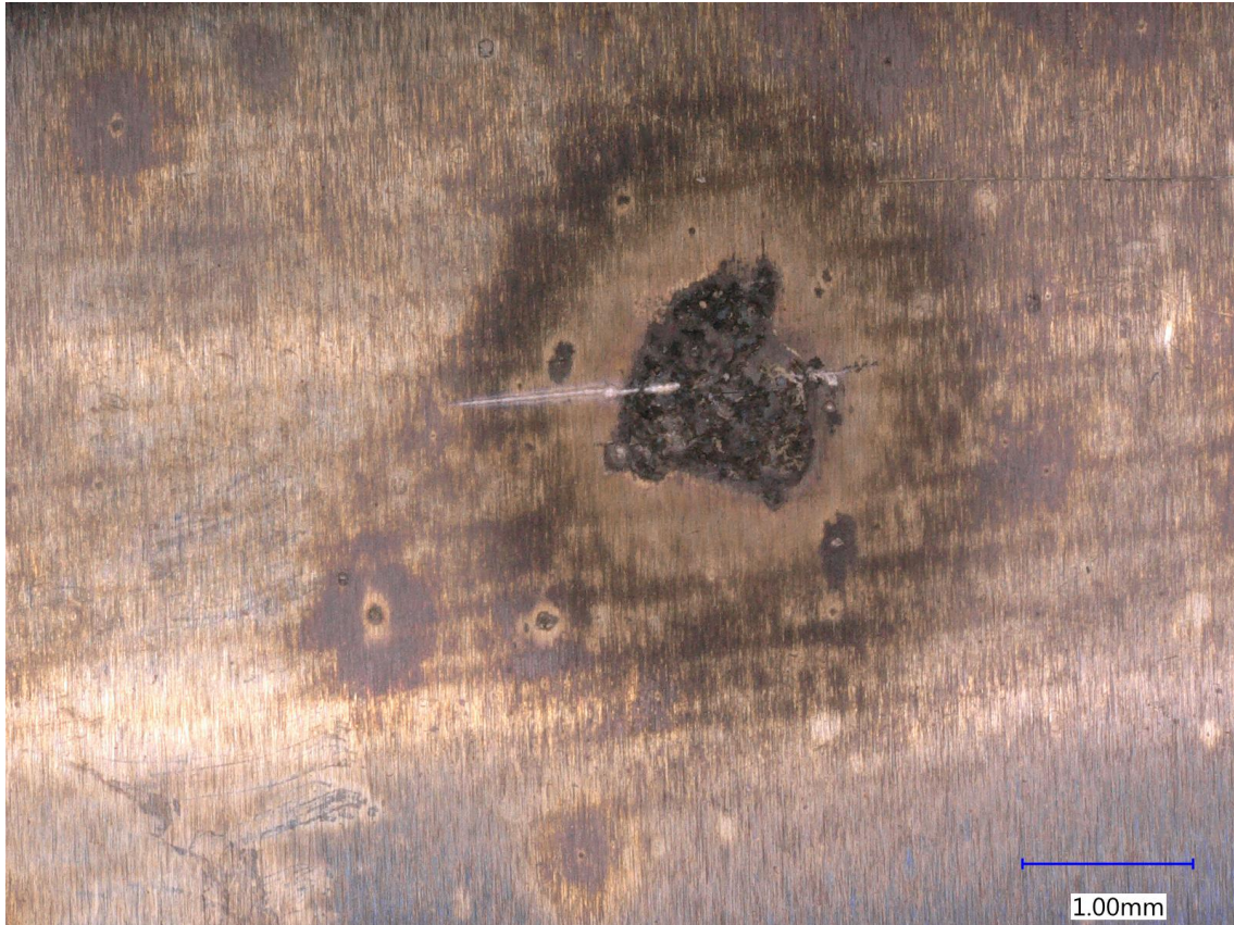
Figure 5.10: An optical image of the 2X salt flux shown above which highlights the crack growing parallel to the dendrite structure
