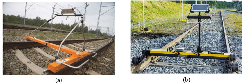
Figure 2. Track geometry inspection trolley: (a) track geometry validation trolley [31]; (b) track geometry inspection trolley with GPS [32].
