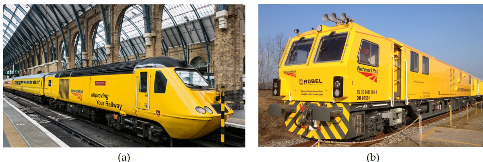
Figure 4. Specially designed train in the UK for railway maintenance: (a) new measurement train (NMT) [41]; (b) mobile maintenance train (MMT) [42].
