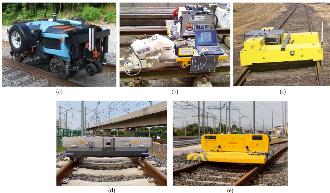
Figure 6. Autonomous track and S&C inspection robot: (a) Railpod [58]; (b) robot with ACFM sensor [59]; (c) AutoScan [48]; (d) RII1005 [22]; (e) Felix [60].
