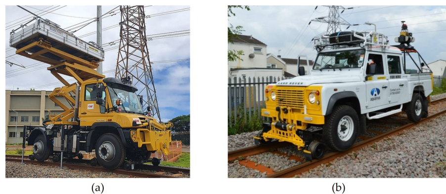
Figure 3. Road–rail vehicles for track maintenance: (a) Unimog road rail vehicle for overhead line maintenance [35]; (b) mobile asset management RRV [34].
