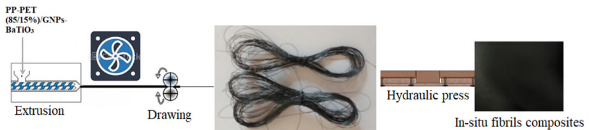
Figure 3-6. Schematic representation of the experimental setup for GNP and Barium titanate(IV) based in-situ fibril Nanocomposites (GBFNC).
