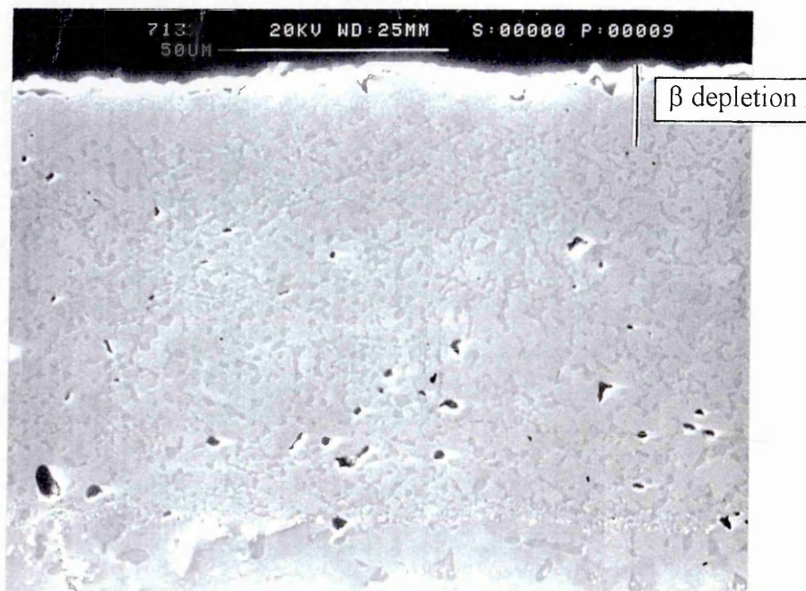
Figure 7.5- \text{H}_2 -10% \text{H}_2\text{O} pre-oxidation, ungritted, aged for 1h at 1150°C
