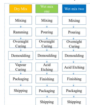
Fig. 3. Cast stone manufacturing process
