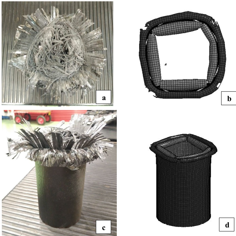
Fig. 12 B60 specimen. Comparison between macroscopic experimental (top view (a), overview (c)) and numerical results (top view (b), overview (d))
