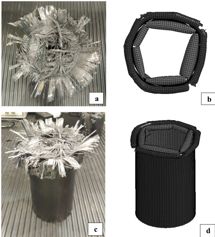
Fig. 13 B30 specimen. Comparison between macroscopic experimental (top view (a), overview (c)) and numerical results (top view (b), overview (d))
