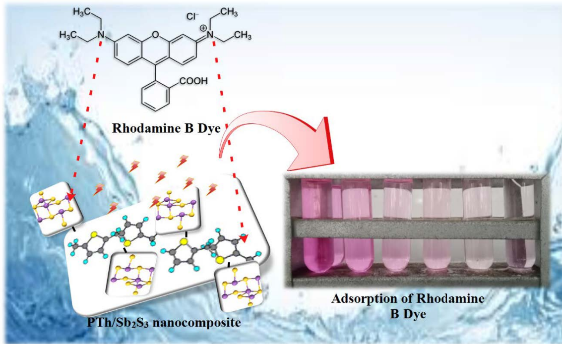
Fig.6. Adsorption mechanism of RhB dye at the surface of PTh/Sb 2 S 3 nanocomposite
