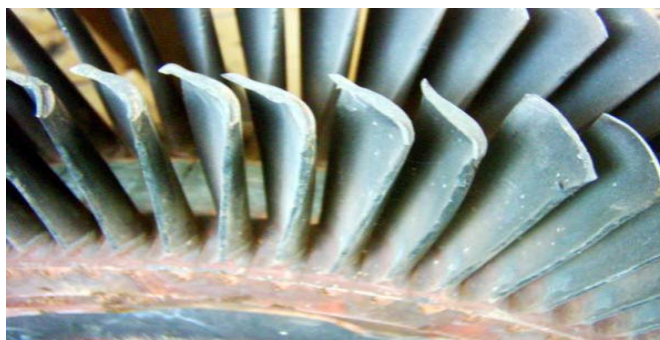
Figure 2-1: Deformed turbine blades under creep attack [95]
