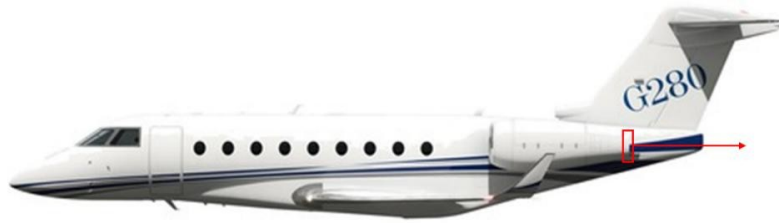
Figure 3.0-2 Gulfstream G280 with rear-fuselage-mounted HTF7250G engines plume aligned with the tailplane [32].
