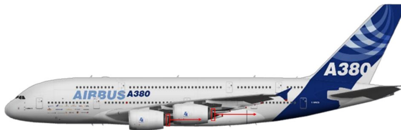
Figure 3.0-3 Airbus A380's Rolls-Royce Trent 900 engines plume spread but exhaust remains directed below the tailplane [33]
