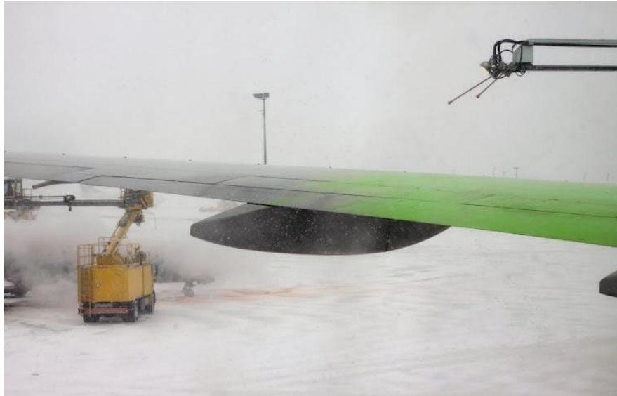
Figure 2.0-4 Type IV fluid applied by operator on the wing of the plane [24]
