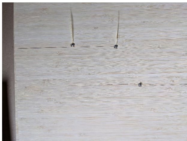
Fig. 6 6 mm Projectile Arrest in Bamboo
