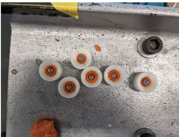
Fig. 3 Gas gun 6 mm ball bearing projectile and 22 mm sabot set-up
