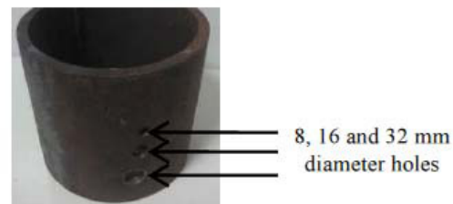
Figure 9: Forged steel round test cylinder.
