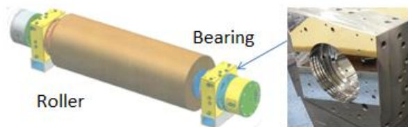
Figure 1. Diamond turned rollers and Hydrostatic bearings & housing.
