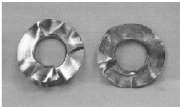
Figure 21. Organometallic polymer-coated (left) and uncoated (right) aluminum fin after 30 days salt spray test in 3.5 wt.% NaCl and 35 °C. No corrosion products developed on the coated component. Reproduced with permission. [122] Copyright 2002, Geothermal Rising.
