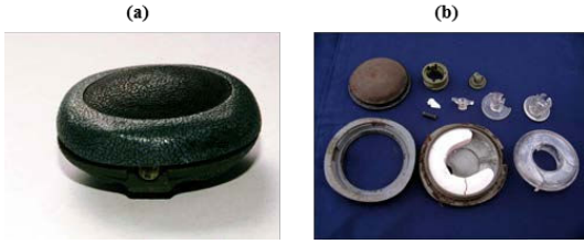
Fig. 8: Neutralised landmine. (a) External view. (b) Disassembled target [11]
